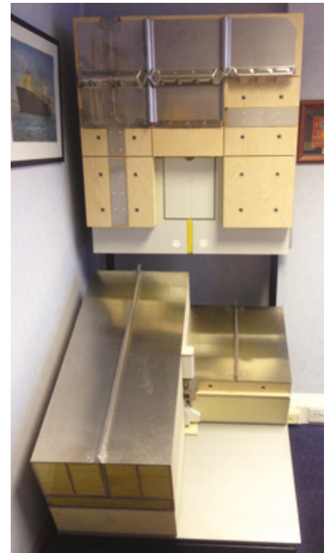
The sections of the GTT No 96 and Mark III membrane tank systems are now a prominent feature of the SIGTTO conference room
