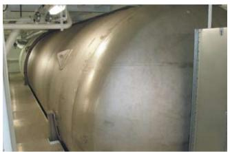
An LNG bunker tank on a Norwegian cross-fjord ferry
