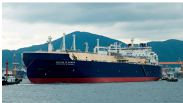
Christophe de Margerie is built to the Arc7 ice class and is the world's first icebreaking LNG carrier
