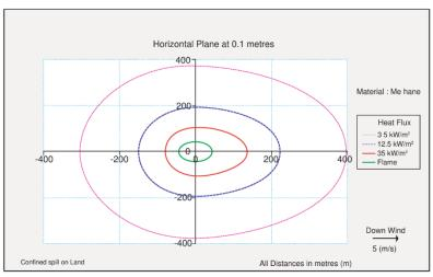
Figure E1: Pool fire analysis of methane showing thermal heat flux
