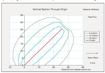
Figure E2: Jet fire analysis of methane showing thermal heat flux
