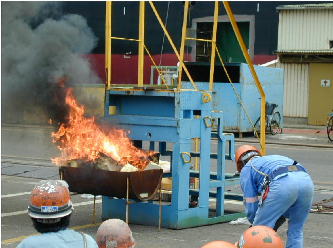
*We then tried it with a small polythene bag on top of the first piece of foam. The bag ignited quickly and the flame seemed to spread in a pool in the foam with a lot of smoke being generated. The fire was extinguished by inverting the foam and letting the liquid (polythene?) pool drop out. The foam then charred and quickly self extinguished.*
