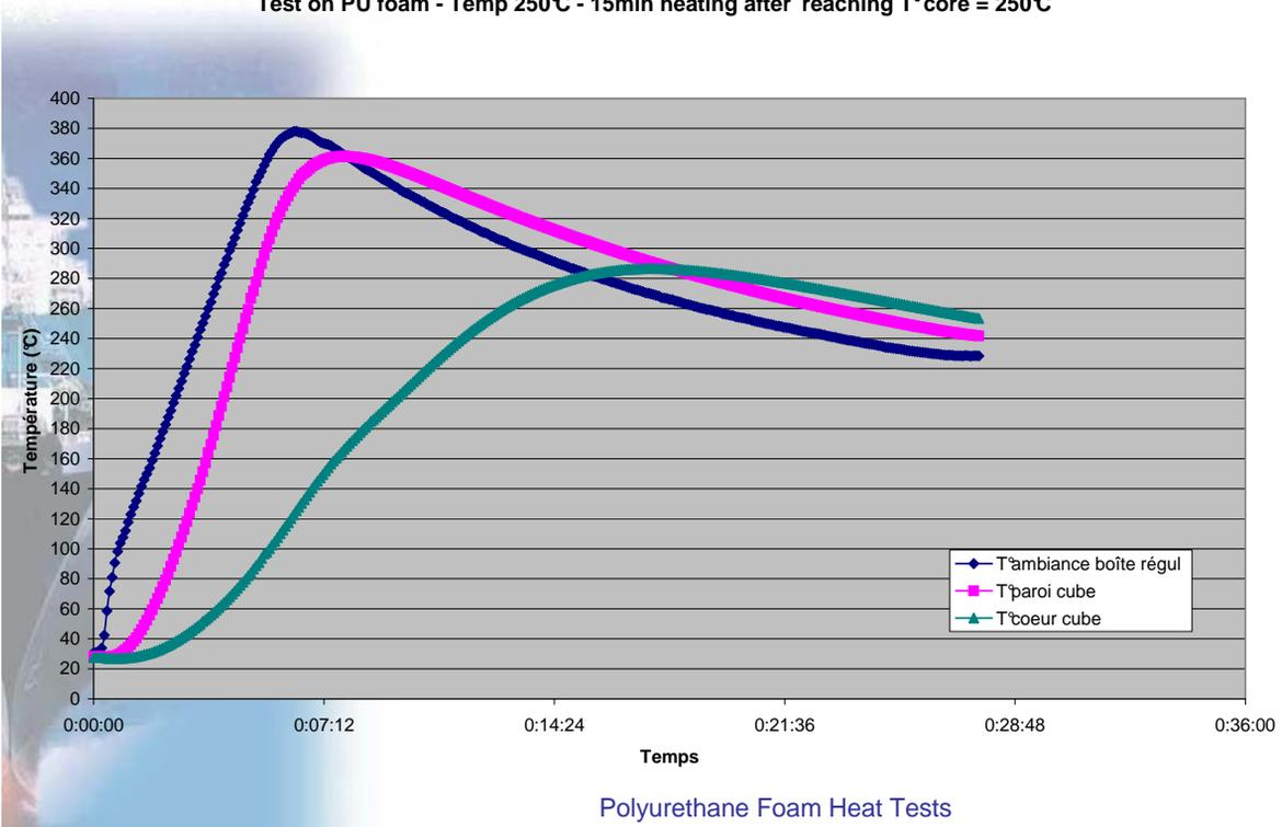
Polyurethane Foam Heat Tests
