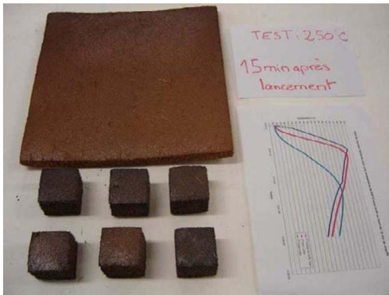
Polyurethane Foam Heat Tests
