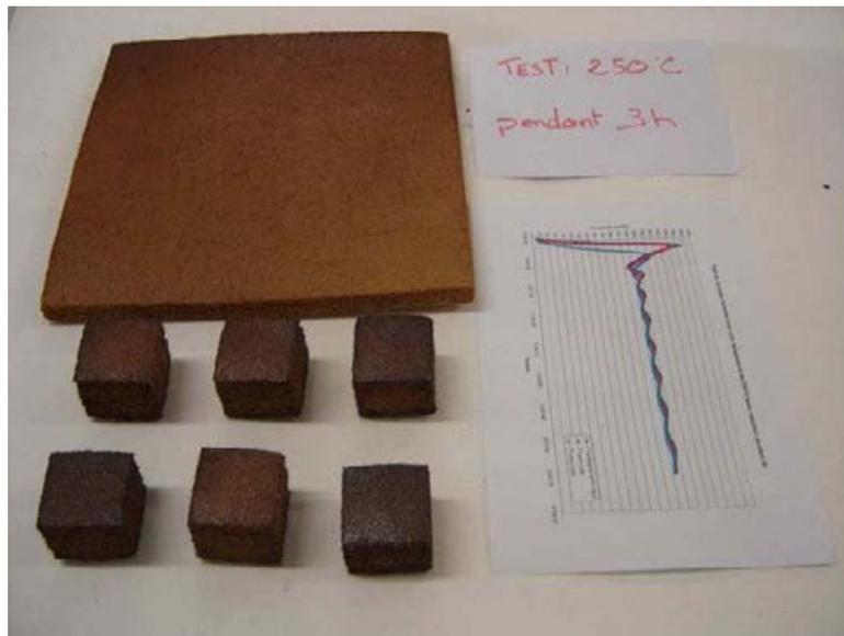
Polyurethane Foam Heat Tests
