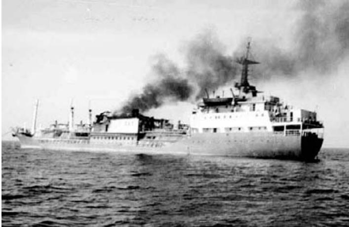
The motor room was so severely damaged that a switch panel was blown onto the deck and cargo pipework outside the room ruptured. In addition, the port and starboard domes of No 3 cargo tank also ruptured. As a result of the explosion the escaping propylene ignited and the fire continued to be fed by cargo evaporating from the damaged domes.
