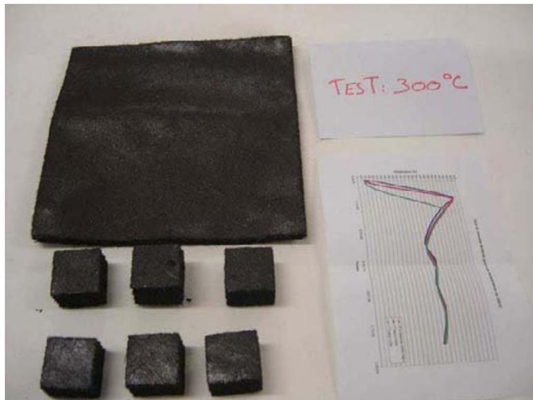
Polyurethane Foam Heat Tests
