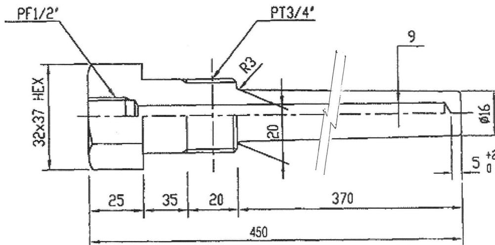
TYPE : DRILLED BAR STOCK, TAPER
