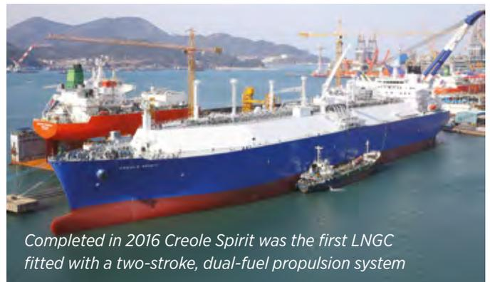
Completed in 2016 *Creole Spirit* was the first LNGC fitted with a two-stroke, dual-fuel propulsion system
