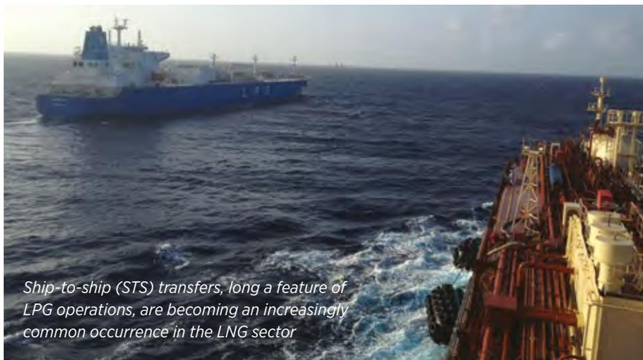
*Ship-to-ship (STS) transfers, long a feature of LPG operations, are becoming an increasingly common occurrence in the LNG sector*
