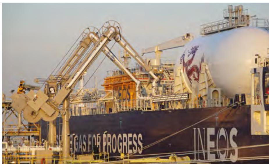
Operated by Evergas, the 27,500 m<sup>3</sup> ethane carrier *Ineos Intrepid* is also able to utilise ethane as a propulsion system fuel
