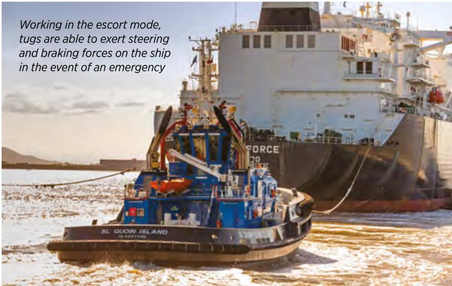
Working in the escort mode, tugs are able to exert steering and braking forces on the ship in the event of an emergency
