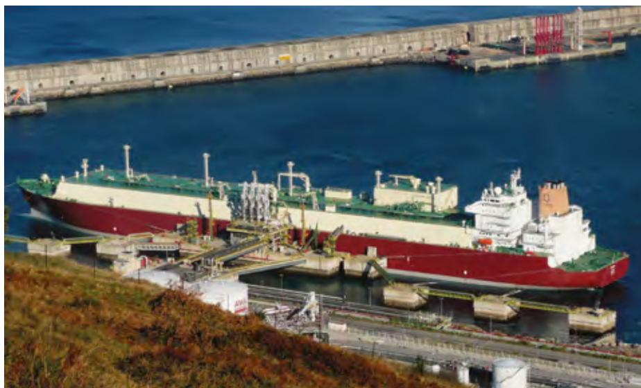
*The nitrogen-cycle reliquefaction systems fitted on Nakilat's Q-flex and Q-max LNG carriers have proved to be effective and advantageous in service*
