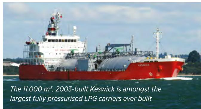
*The 11,000 m<sup>3</sup>, 2003-built Keswick is amongst the largest fully pressurised LPG carriers ever built*
