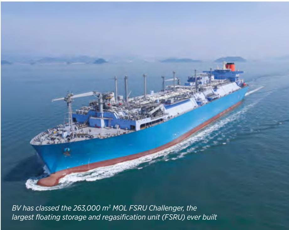
BV has classed the 263,000 m<sup>3</sup> MOL FSRU Challenger, the largest floating storage and regasification unit (FSRU) ever built
